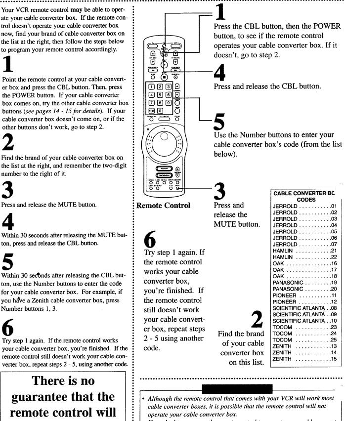
• If you had to program the remote control to operate your cable converter box here, whenever you replace the batteries in the remote control, you will have to program the remote control again.
